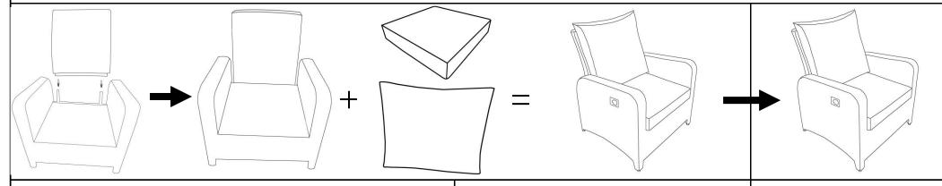
Step 1. Take out all the components and place them onto a soft and clean surface. Put the recliner seat (A) in its upright position. Hold up the recliner back (B) and aim the tubes located at the underside of the backrest, and plug-slot into the 02 tubes which are on the seat base. Push firmly and fully downwards.
