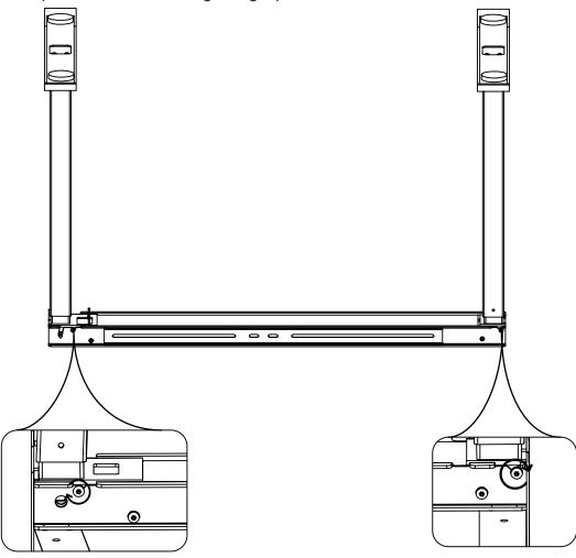
Tighten the screws for the foot. And don't forget tighten the folding legs.
