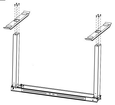
Open the frame to the right angle position. Assemble the base.
