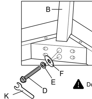
⚠ Do not fully tighten the hardware.
