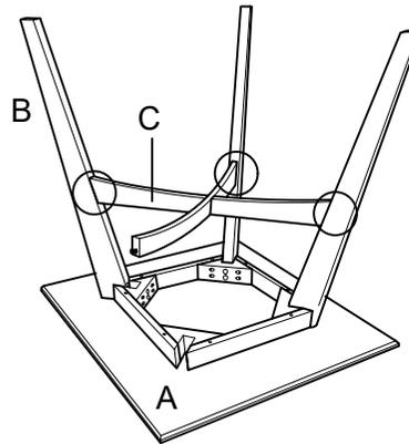
⚠ Do not fully tighten the hardware.
