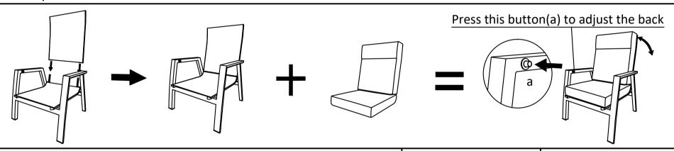
Step 1. Take out all the components and place them onto a soft and clean surface.put the recliner seat(A) in its upright position. Hold up the recliner (C)onto the chair, as back(B)and aim the tubes located at the underside of the backrest, and Plug-slot into the 02 tubes which are on the seat base. Push firmly and fully downwards
